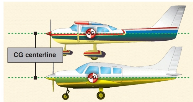
Figure 1.36 Keel area for lateral stability
