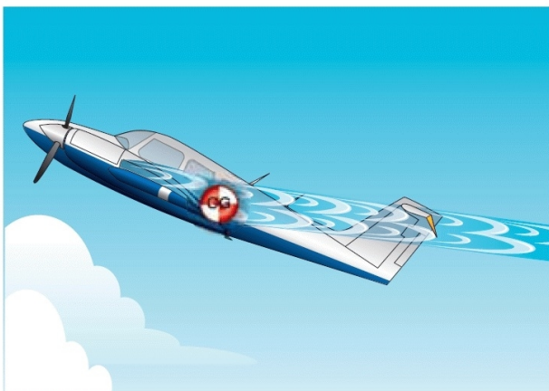
Figure 1.74 Aeroplane with a T-tail design at high AOA and an aft CG
