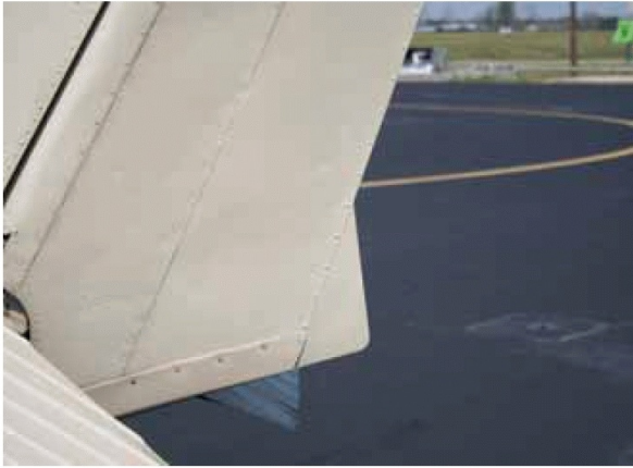
Figure 1.85 A ground adjustable tab is used on the rudder of many small aeroplanes to correct for a tendency to fly with the fuselage slightly misaligned with the relative wind
