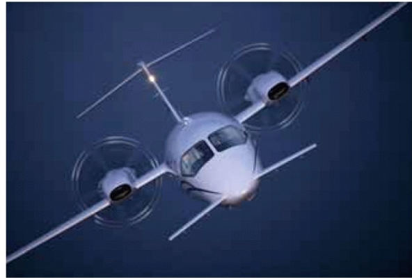
Figure 1.77 The Piaggio P180 with a variable sweep canard design which provides longitudinal stability about the lateral axis
