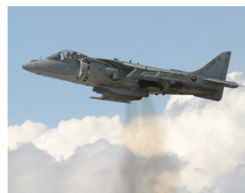
Figure 1.14 Some aircraft can change the direction of thrust
