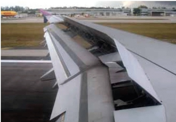
Figure 1.82 Spoilers reduce lift and increase drag during descent and landing
